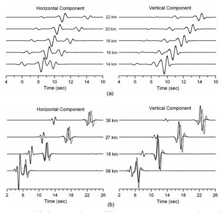
**Figures 6a and 6b.** Comparison of computed FD responses using stress imaging technique (dotted line) and VGR-stress imaging technique (solid line) at different epicentral distances using a deep source and a shallow source, respectively.
