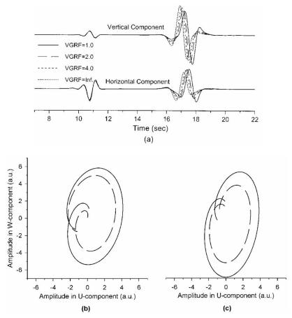
**Figures 7a-7c.** Comparison of computed response at an epicentral distance of 27.0 km using different VGRF; and shape of the particle motion trajectory at epicentral distances of 18 km (solid line) and 36 km (dotted line) using (b) stress imaging technique) and (c) VGR-stress imaging technique for VGRF =  $10^7$  (Note: a.u. means arbitrary unit).
