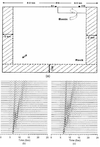
Figures 8a to 8c. shows the basin-edge model and b & c show the horizontal components of the responses computed using uniform grid and a variable size of a grid cell.
