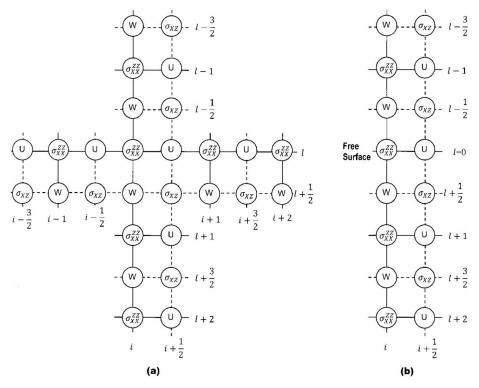
**Figure 1a.** Staggering technique for P-SV wave modeling with fourth order spatial accuracy. Particle displacement and density are defined the midway between two adjacent grid points in the horizontal and vertical directions. Normal stress components and Lame's parameters are defined at grid nodes and shear stress component and modulus of rigidity are defined at the centre of the grid cell; and **1b**. extended grid points above the free surface.
