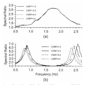
**Figure 5.** A comparison of variation of fundamental frequency and higher modes of resonance frequency of soil layer with VGRF in case of source dominated by P-wave (using vertical component) and S-wave (using horizontal component), respectively. (Note: considered thickness of soil in Figures 5a and 5b were 180 m and 120m, respectively).
