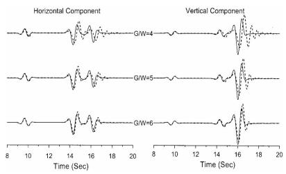
**Figure 2.** Comparison of computed responses of a homogeneous half-space model using different number of grid points per shortest wavelength (G/W) with the response computed using 12 grid points per-shorted wavelength.
